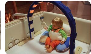
The arched gym is a structure that can be placed in the CareToy H where toys can be hung in the three points of interest. Twelve different **orange lights** are embedded into the arch that progressively switch on and off from one side to the middle and/or to the other side.
