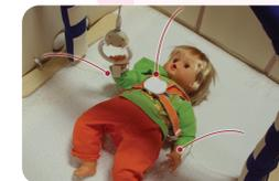
In order to get some informations about the arms and trunk movements ST Microelectronics (CareToy partner) developed **wireless magneto-inertial wearable devices** designed as bracelets and chest strap.
